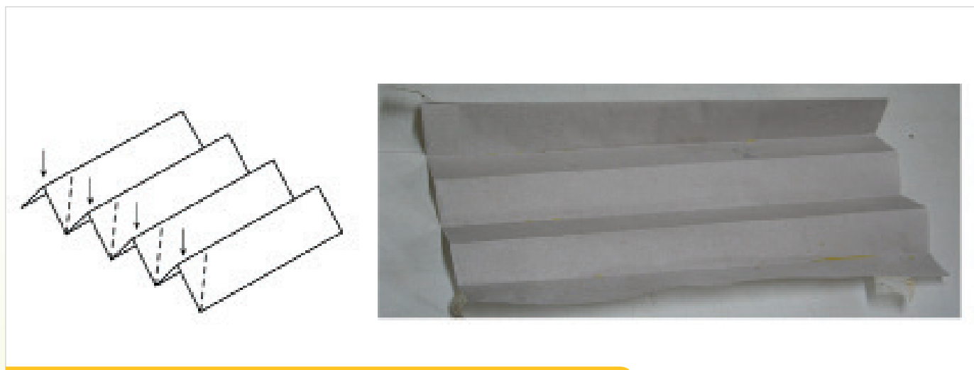
Figure 25: Cut pieces of butter paper (40 cm W x 50 cm L) are folded in accordion form
