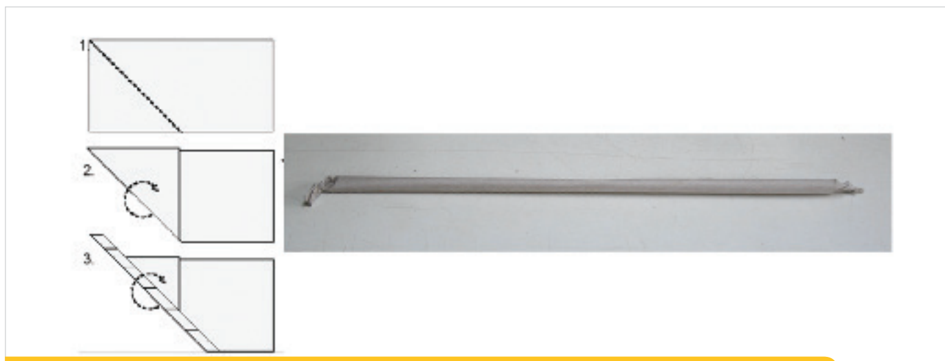
Figure 24: Cut pieces of butter paper (6 cm W x 75 cm L) are wound spirally, with each end twisted to hold the spirals firm.
